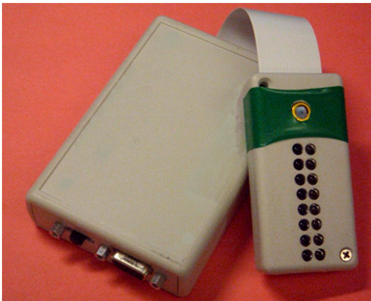
Figure 4-14 Current NIRS System (Data Acquisition Unit, left, with Optical Module)
